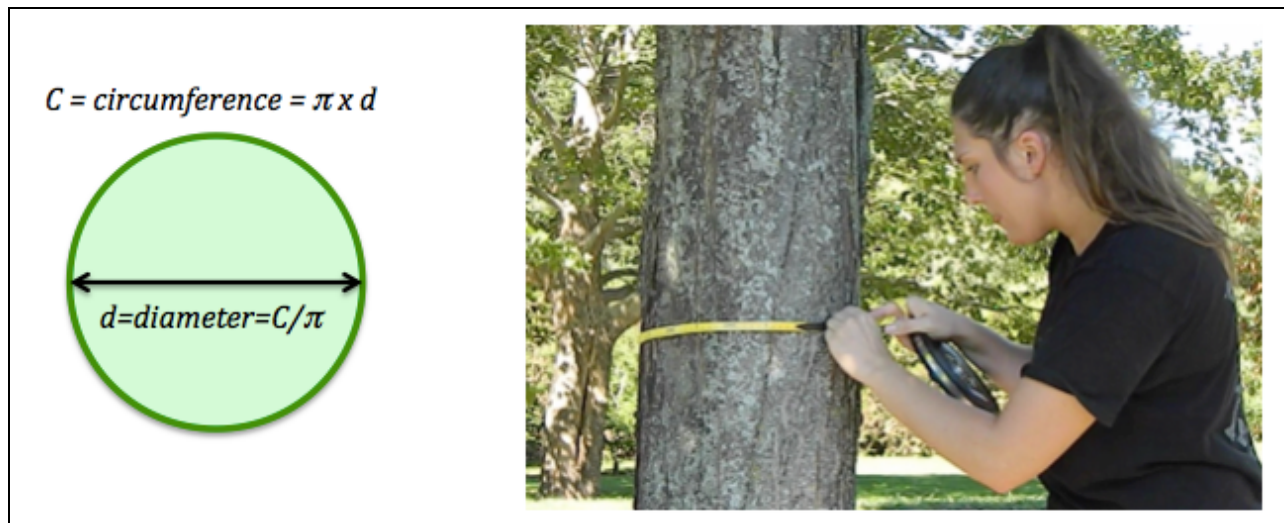
Figure 2: The circumference and diameter of a circle are related by the factor pi: \pi=3.14159 . Measure the circumference of the tree (photo) in order to calculate the diameter.
